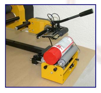
The CP21-LC system will wrap labels up to 95mm wide (including backing paper) around the circumference of cylindrical products. Products are placed on the drive rollers and the applicator beak is lowered using the hand lever starting labelling automatically.
